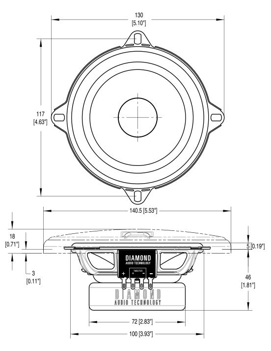
M351, M351i General dimensions in millimeters and [inches]. Not to scale.
